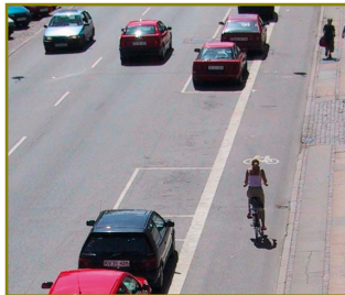
Cycle paths are always placed between parked cars and the footpath. Cycle paths are one way and on each side of the street. Copenhagen, Denmark
