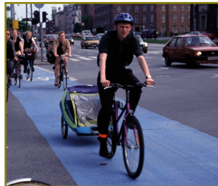
Marked lanes: In most intersections, especially more complex ones, the cycle lane is marked in the paving so it is clear which space belongs to whom. Paris, France - Copenhagen, Denmark
